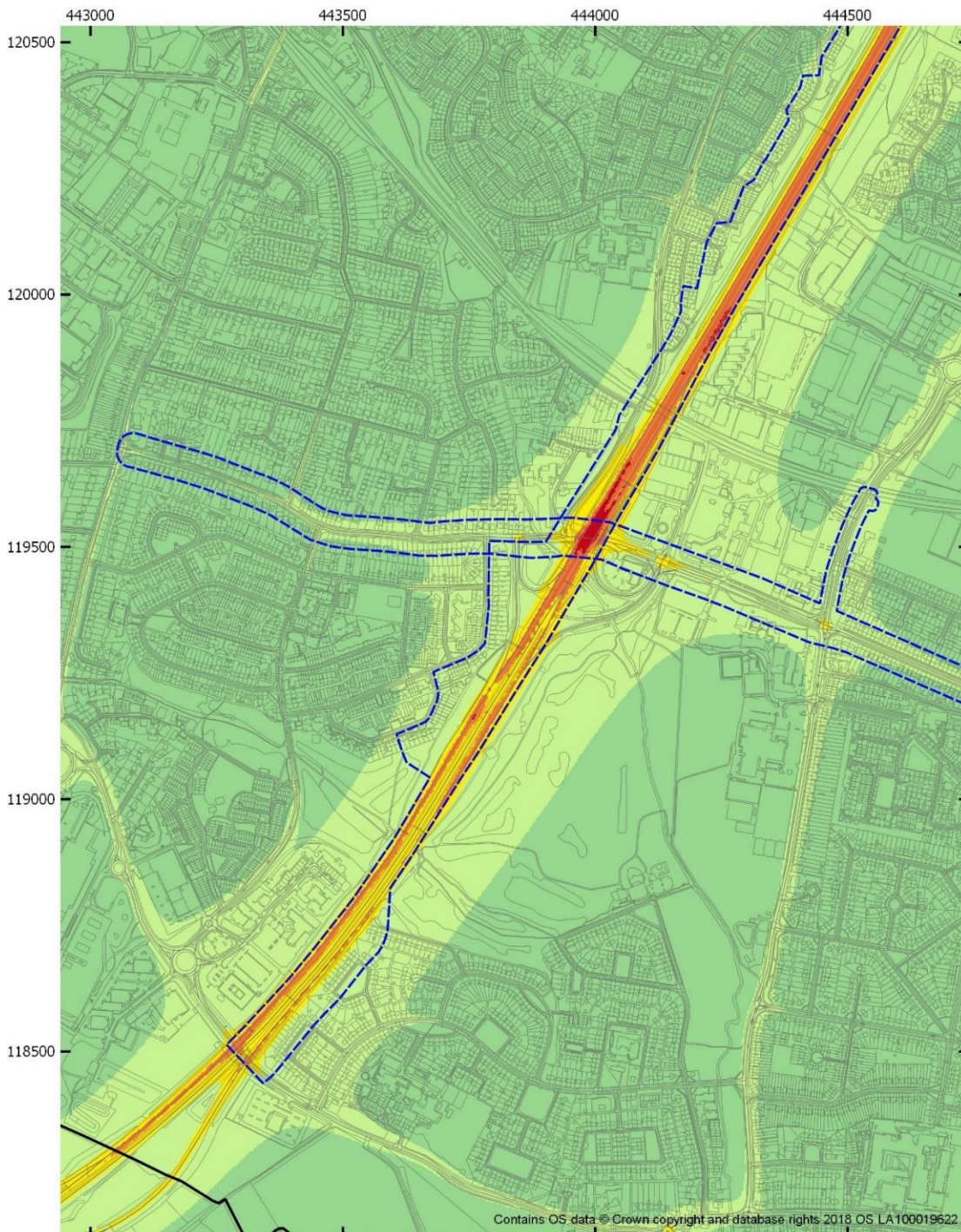
Figure 4-16 Annual mean PM 10 concentration model results for 2020 No New Traffic Interventions (2020 NNTI) scenario - AQMA No. 1 (A335 / Eastleigh) (West)
