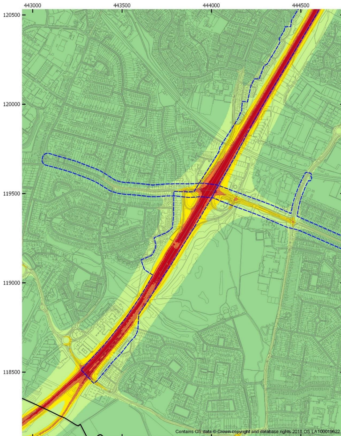
Figure 4-48 Short-term PM 10 concentration model results for 2020 No New Traffic Interventions (2020 NNTI) scenario - AQMA No. 1 (A335 / Eastleigh) (West)
