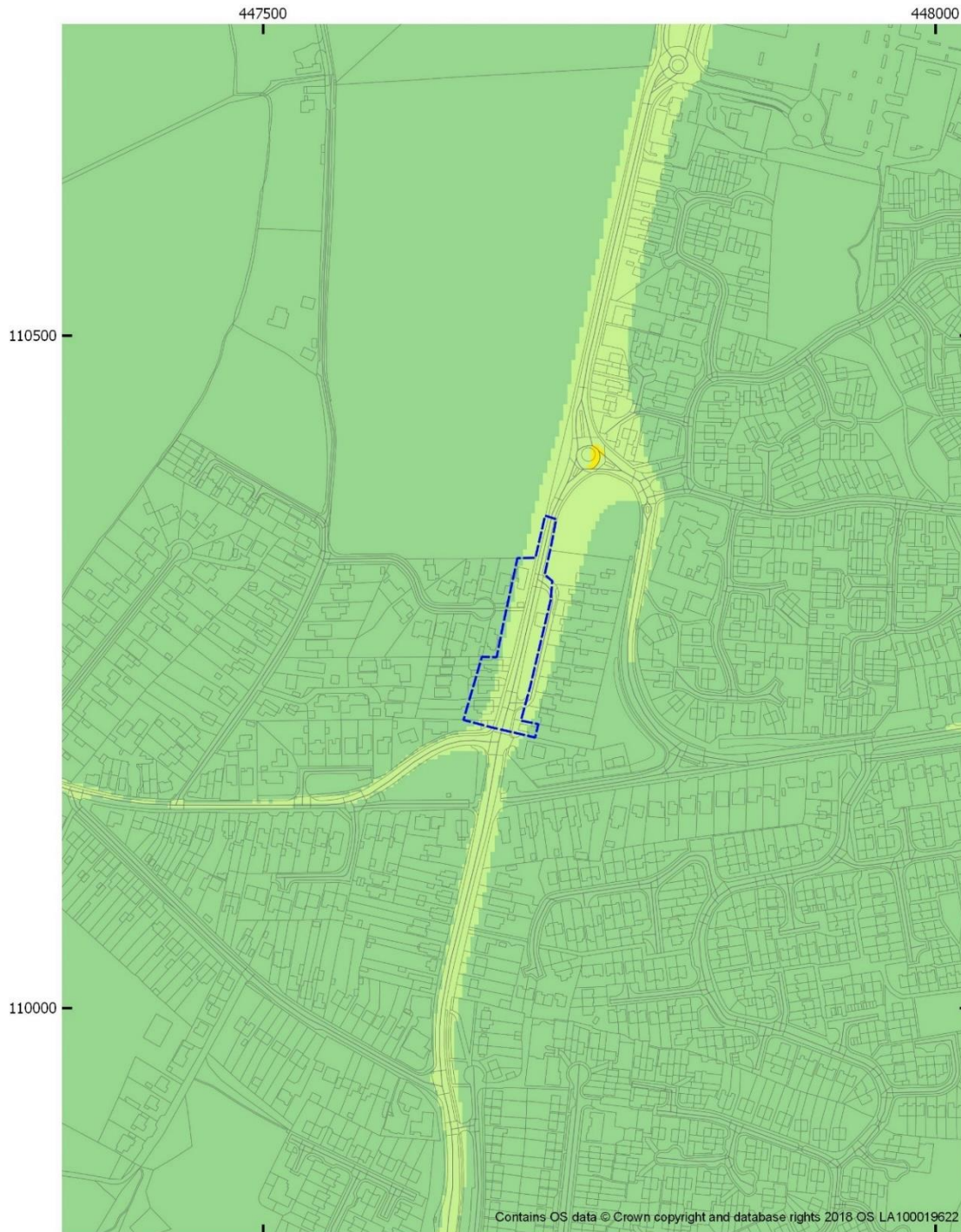
Figure 4-27 Annual mean PM 10 concentration model results for 2020 With Interventions (2020 WI) scenario - AQMA No. 3 (Hamble Lane)
