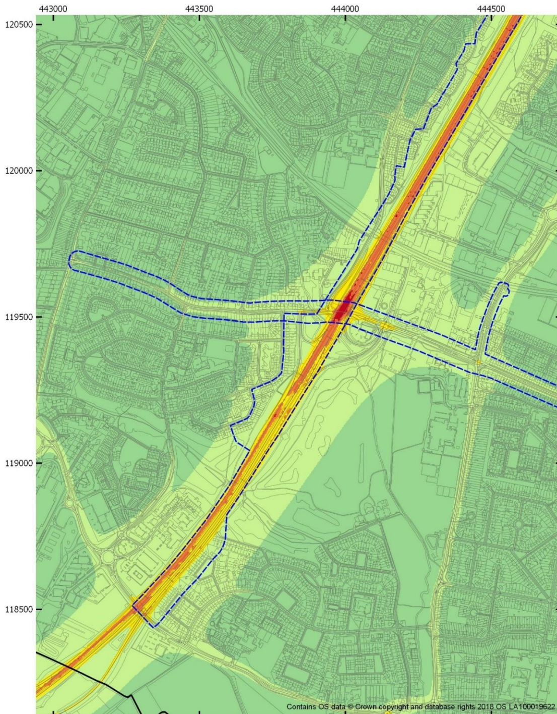
Figure 4-15 Annual mean PM 10 concentration model results for 2020 With Interventions (2020 WI) scenario - AQMA No. 1 (A335 / Eastleigh) (West)
