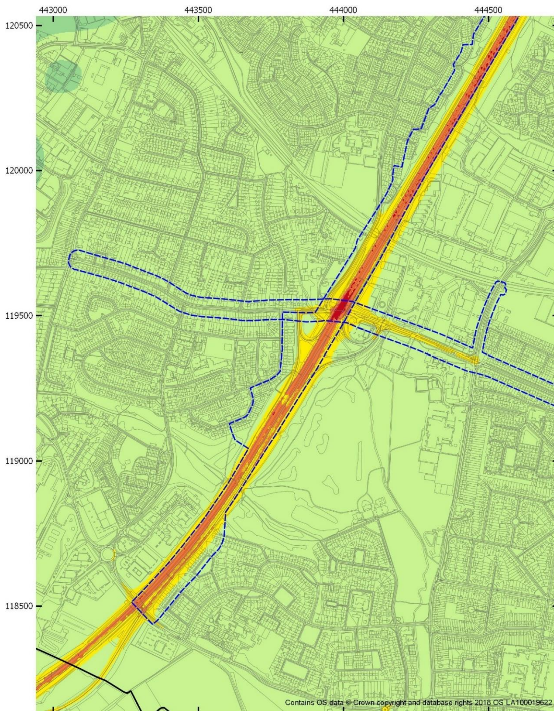
Figure 4-17 Annual mean PM 2.5 concentration model results for 2020 With Interventions (2020 WI) scenario - AQMA No. 1 (A335 / Eastleigh) (West)
