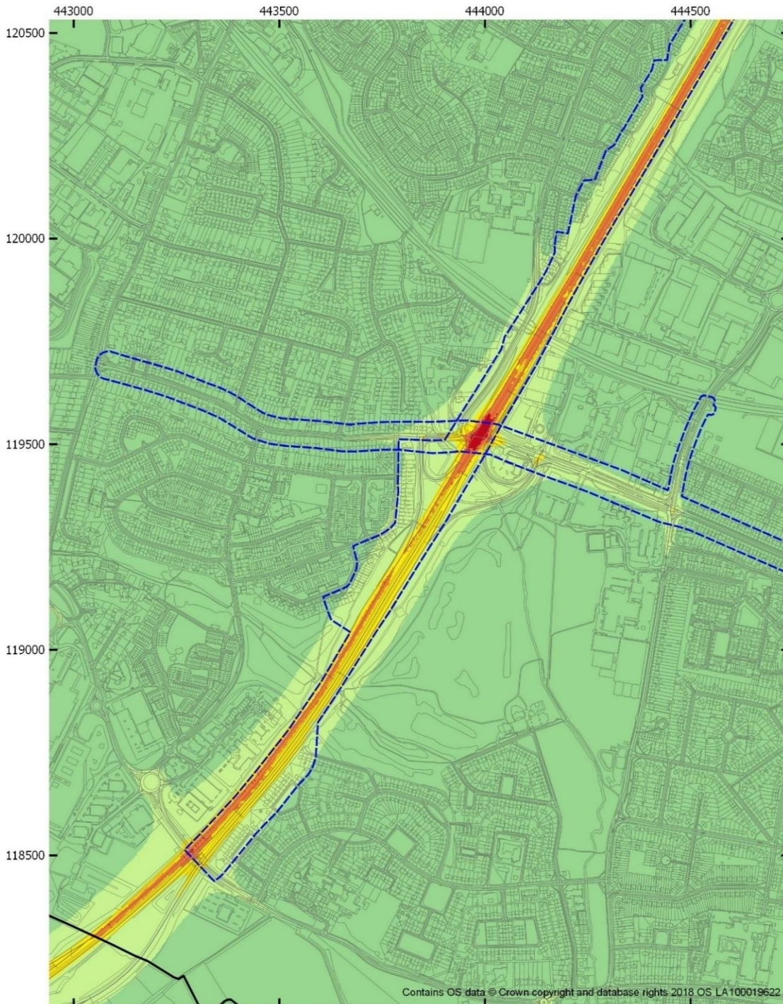
Figure 4-46 Short-term NO 2 concentration model results for 2020 No New Traffic Interventions (2020 NNTI) scenario - AQMA No. 1 (A335 / Eastleigh) (West)
