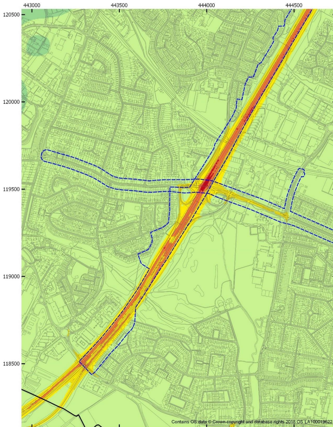
Figure 4-18 Annual mean PM 2.5 concentration model results for 2020 No New Traffic Interventions (2020 NNTI) scenario - AQMA No. 1 (A335 / Eastleigh) (West)
