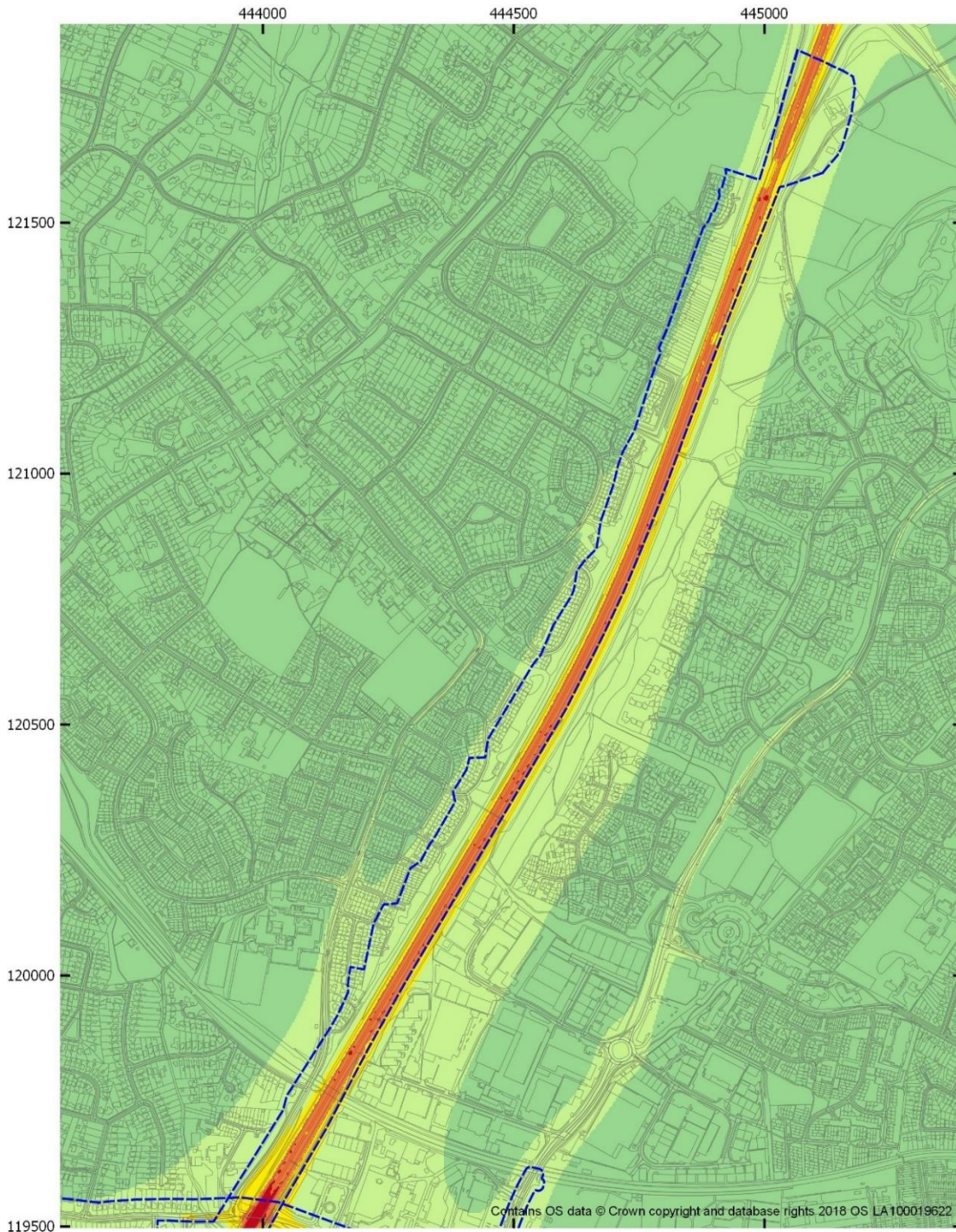
Figure 4-21 Annual mean PM 10 concentration model results for 2020 With Interventions (2020 WI) scenario - AQMA No. 2 (M3) (North)
