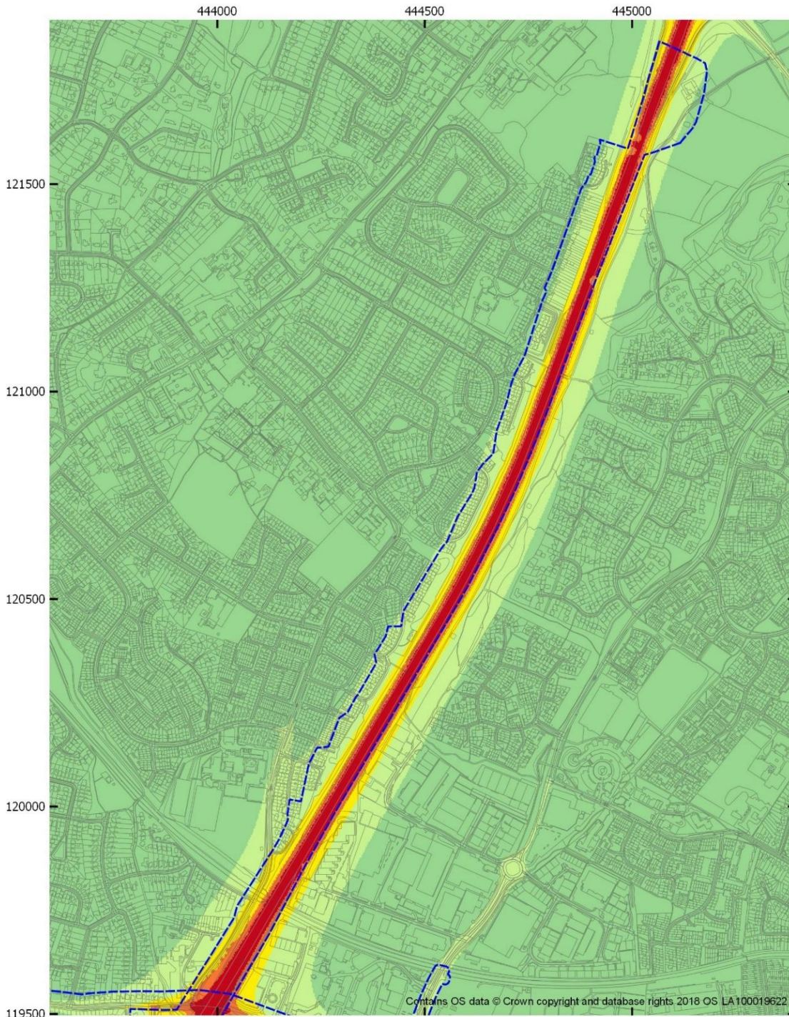
Figure 4-51 Short-term PM 10 concentration model results for 2020 With Interventions (2020 WI) scenario - AQMA No. 2 (M3) (North)
