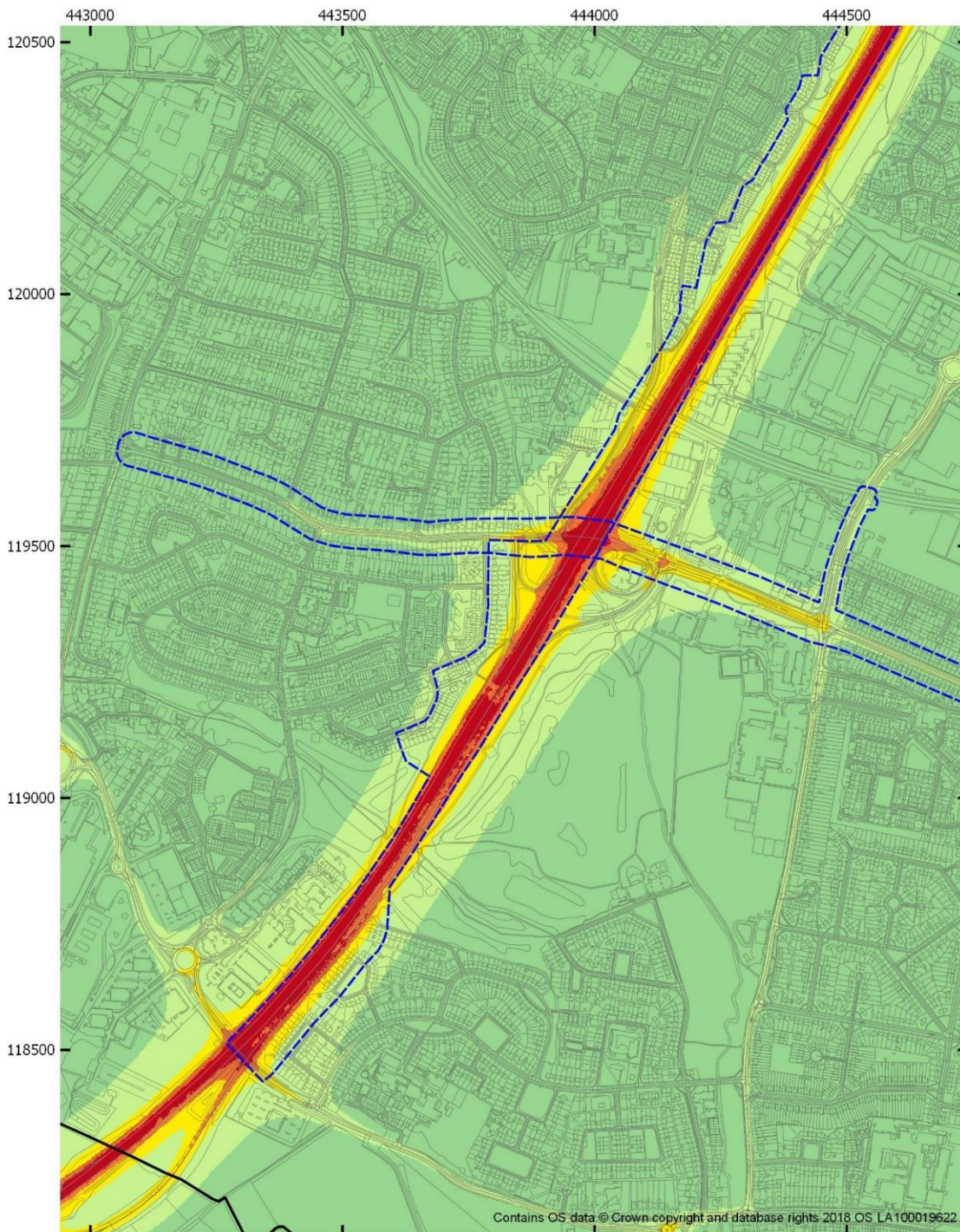
Figure 4-47 Short-term PM 10 concentration model results for 2020 With Interventions (2020 WI) scenario - AQMA No. 1 (A335 / Eastleigh) (West)
