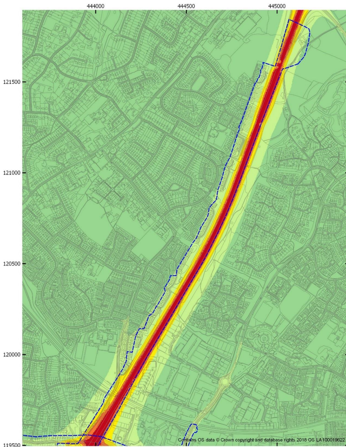
Figure 4-52 Short-term PM 10 concentration model results for 2020 No New Traffic Interventions (2020 NNTI) scenario - AQMA No. 2 (M3) (North)
