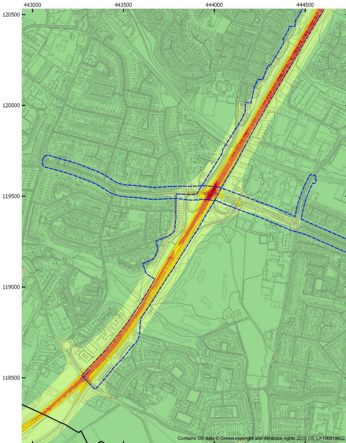
Figure 4-45 Short-term NO 2 concentration model results for 2020 With Interventions (2020 WI) scenario - AQMA No. 1 (A335 / Eastleigh) (West)
