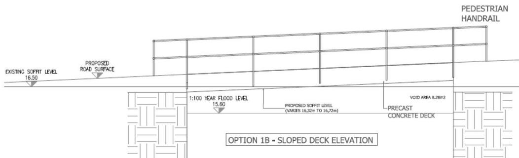
Option 1B provides optimum void space beneath the bridge, whilst also satisfying the parameters set out with regards to the road and flood levels. Moreover, the design incorporates the use of handrails instead of the existing concrete parapets provides ecological benefits to the surrounding area, facilitating the passage of light through the bridge section and minimising shading influences on the local ecology.
