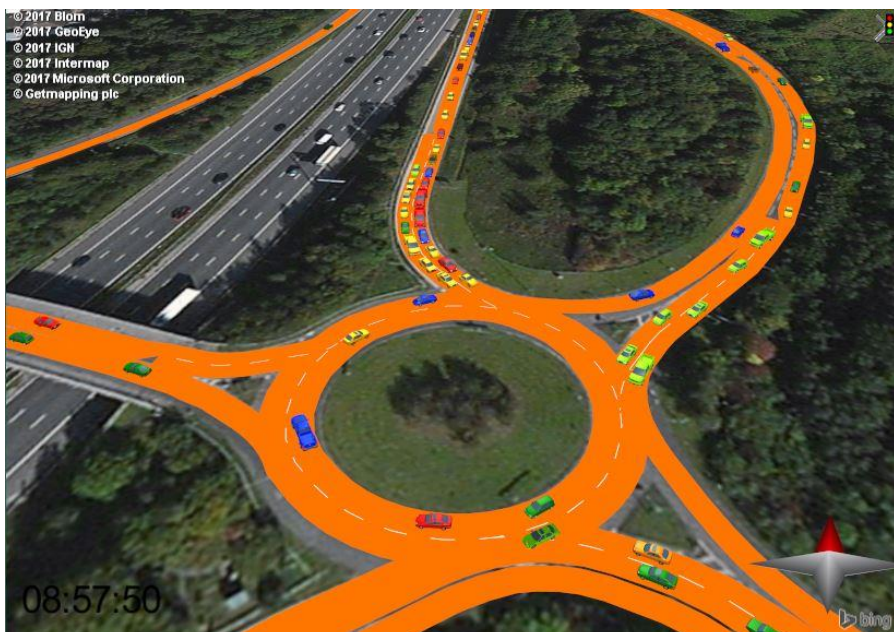
Figure 6-4 J3 – DS Option 4 creates long queues on the M3 off-slip (AM Peak)
