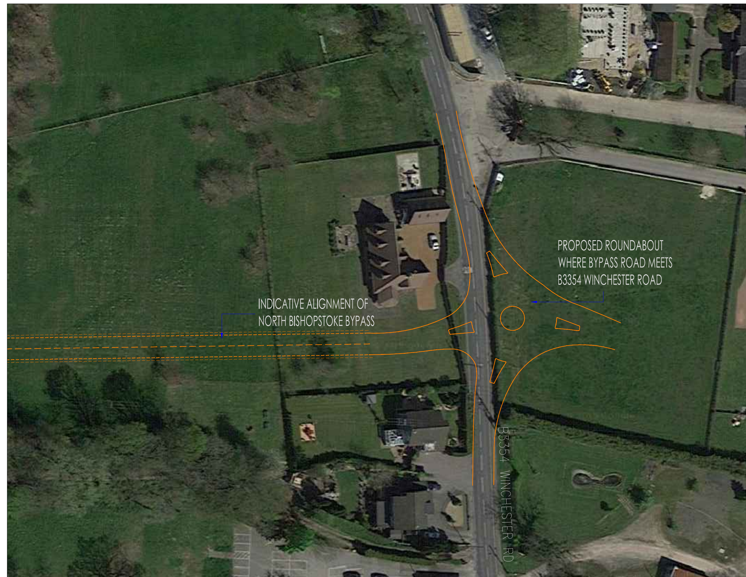
INSET 4 - PROPOSED ROUNDABOUT AT B3354 WINCHESTER ROAD
