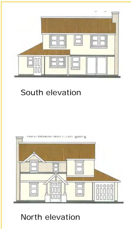
Optimised glazing areas to maximise the benefits of passive solar design, whilst maintaining a conventional appearance (The Concrete Centre)
