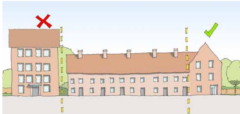
Fig.12: New development should generally not be more than 1 storey higher where it directly adjoins or is close to existing residential development.
