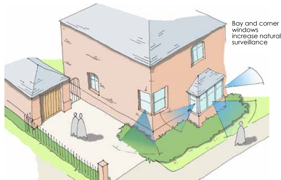
Fig.81: Corner rooms should have windows in walls addressing both sides of the street to allow complete surveillance and avoid the problem of blank flank walls.
